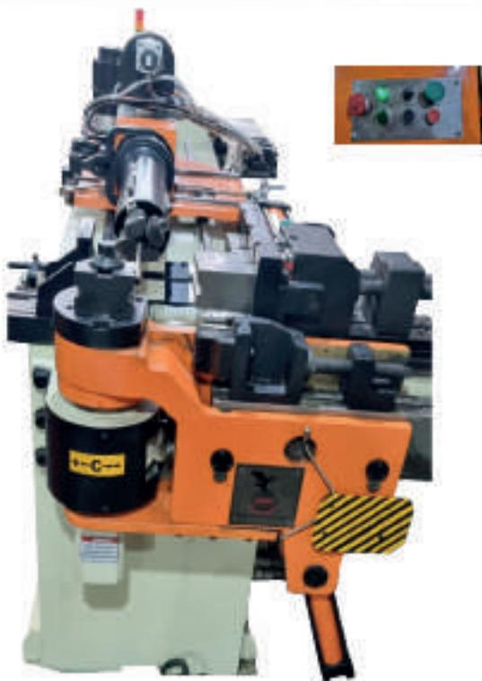
Double Axis CNC Pipe Bending Machine means that we have 3 Axis to perform one is bending and another one will be linear positional axis which is operated by electric servo motor & Third Axis will perform to rotate the pipe.
