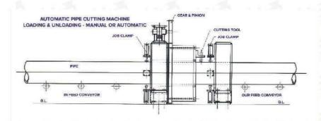
CUTTING RANGE diameter of 76 to 163 mm PRODUCTION: 300 - 400 PC / 12 Hours MOTOR: 10 HP
