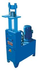
This Machine Can be used for bulk production of air conditioner hoses with Aluminium caps, The rubber moulded dies are openable which enables hoses having complex shapes to be crimped. The crimping depth can be adjusted by a micrometer having an accuracy of 0.05 mm. This machine is supplied with 3 sets of dies. Extra dies are also available on demand.
