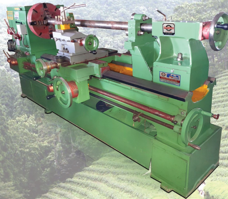
Lathe Machine with Chasing attachment
